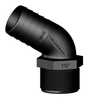
TruDesign Tails are moulded from a glass reinforced nylon composite. High strength, high-modulus glass fibres impregnated into the nylon provides dramatic strength, stiffness, toughness, and dimensional stability. TruDesign Tails eliminate the corrosion and electrical bonding problems associated with metallic fittings. The Tails are designed for twin hose clamps, and to not crush under high load conditions.
